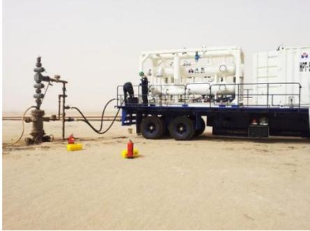
Haimo [High Performance Tester](#) (HPT) is an excellent tool for field verification of meters including MPFM.
